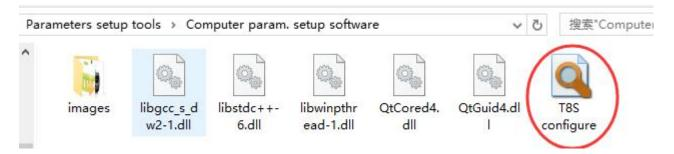
Choose Port Number( COM port will be automatic identified when connected), setting baud rate: **115200**, **8-1-None**(8 data bits, 1 stop bit, no parity check), click OPEN to connect.
